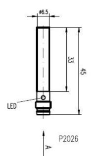
**Inductive Sensors** BES 516-371-G-E5-C-S 49 D6.5 x 45 normally-open Sn=2mm shielded
